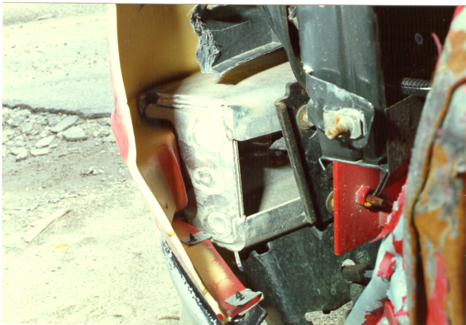
Left Corner Of The Front Bumper Reinforcement Bar.
